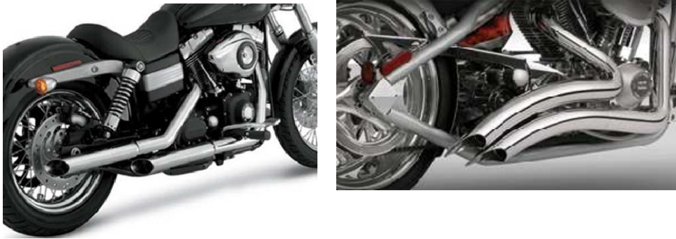
FIGURE 4-1. Exhaust systems that appear to have little or no muffling installed. Obtained from Internet post-roundtable.
