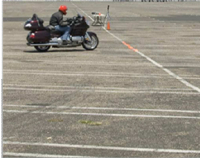
FIGURE 2-1. A motorcycle undergoing the EPA noise test procedure. Photo presented at roundtable by the Motorcycle Industry Council.
